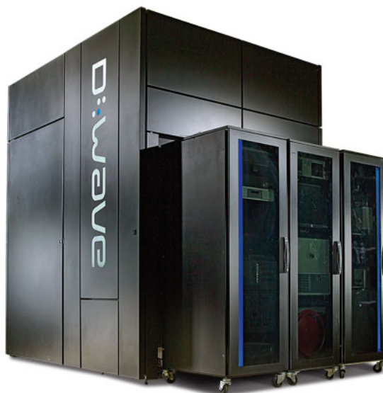
Figure 1.5: The D-Wave architecture is based on superconducting qubits. The first version was a 128-qubit processor, superseded in 2013 by a 512-qubit processor. Whether this quantum annealer outperforms classical computers is source of debate.
