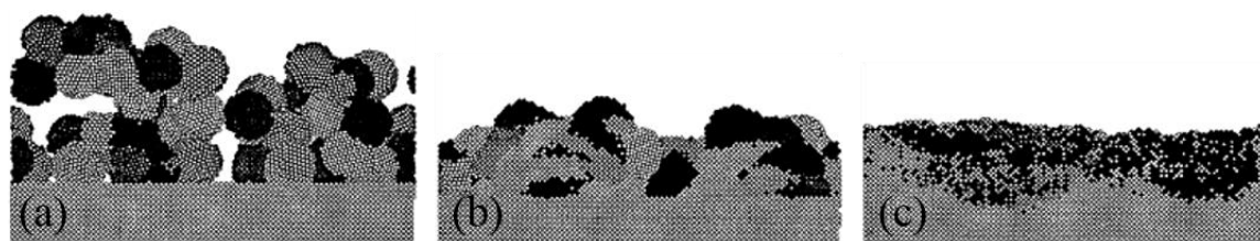
Fig. 21: Molecular-dynamics simulations of the morphology of films obtained by Mo 1043 cluster deposition on a Mo(001) surface as a function of the cluster incident kinetic energy: (a) 0.1 eV/atom; (b,) 1 eV/atom; (c) 10 eV/atom 20 .
