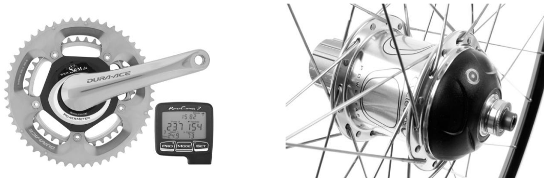
Figure 8. Pictures show two instruments for the measure of the \dot{W}_{EXT} in cycling, the SRM powermeter (a) and the PowerTap (b).
