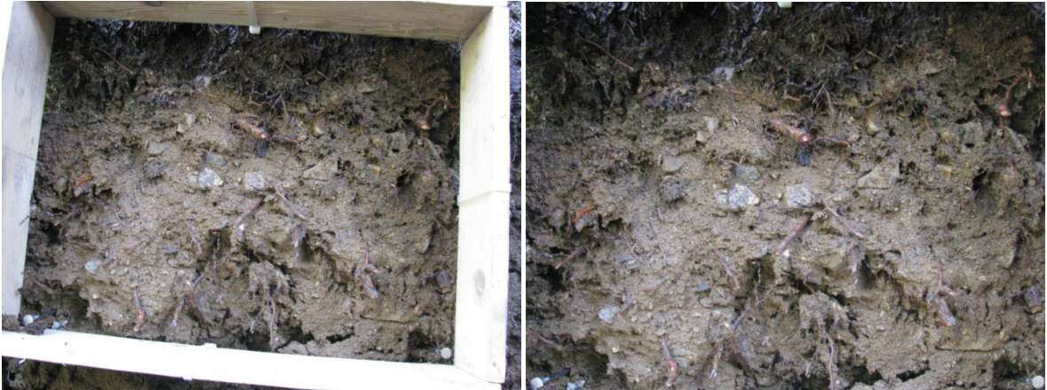
Fig. B 13 Example of applied frame and corresponding rectified picture, trench in undisturbed forest, Averara.
