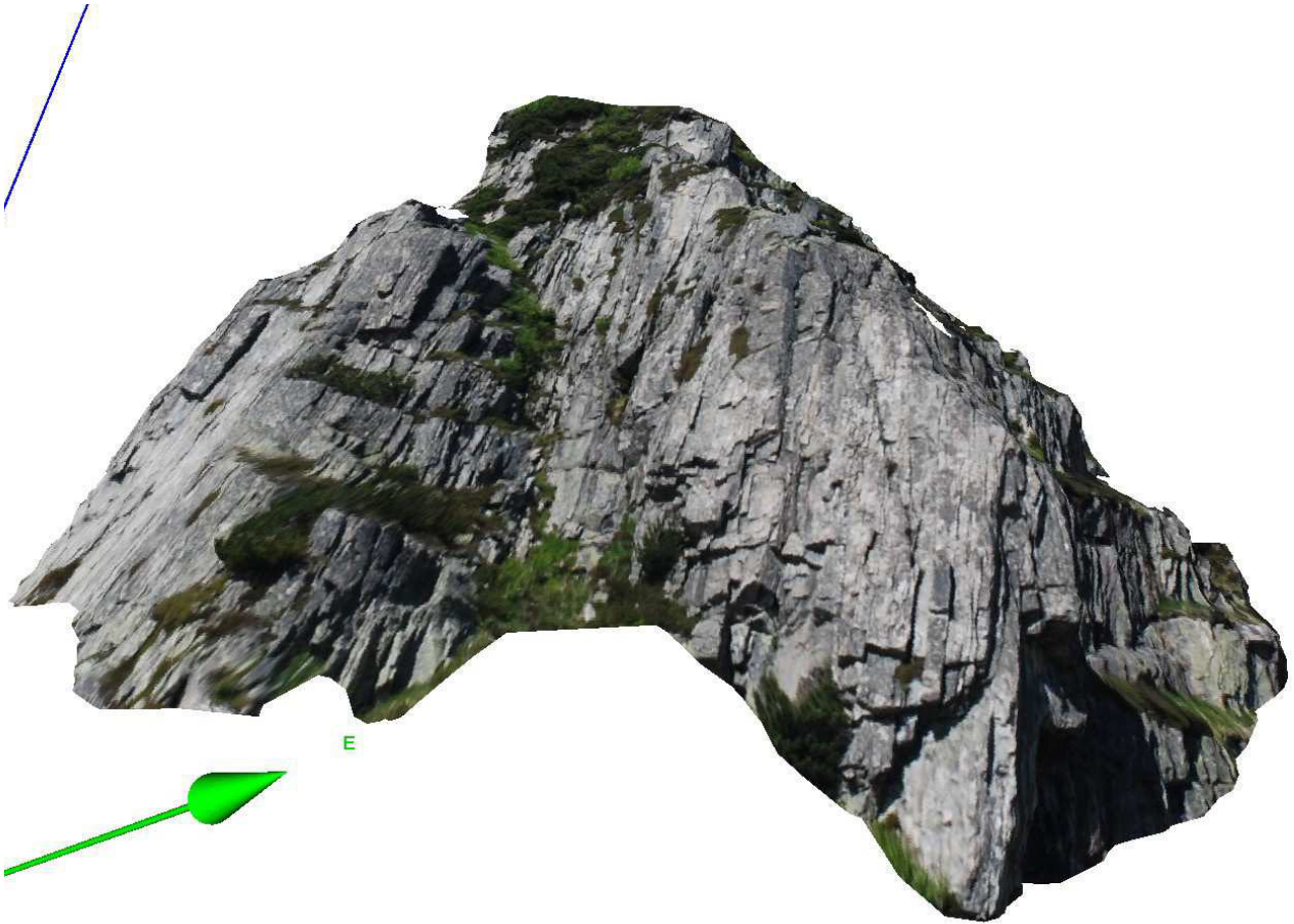
Figure 54 – Example of photogrammetric model with exfoliation joints belonging to generation 1 (model n°28)
