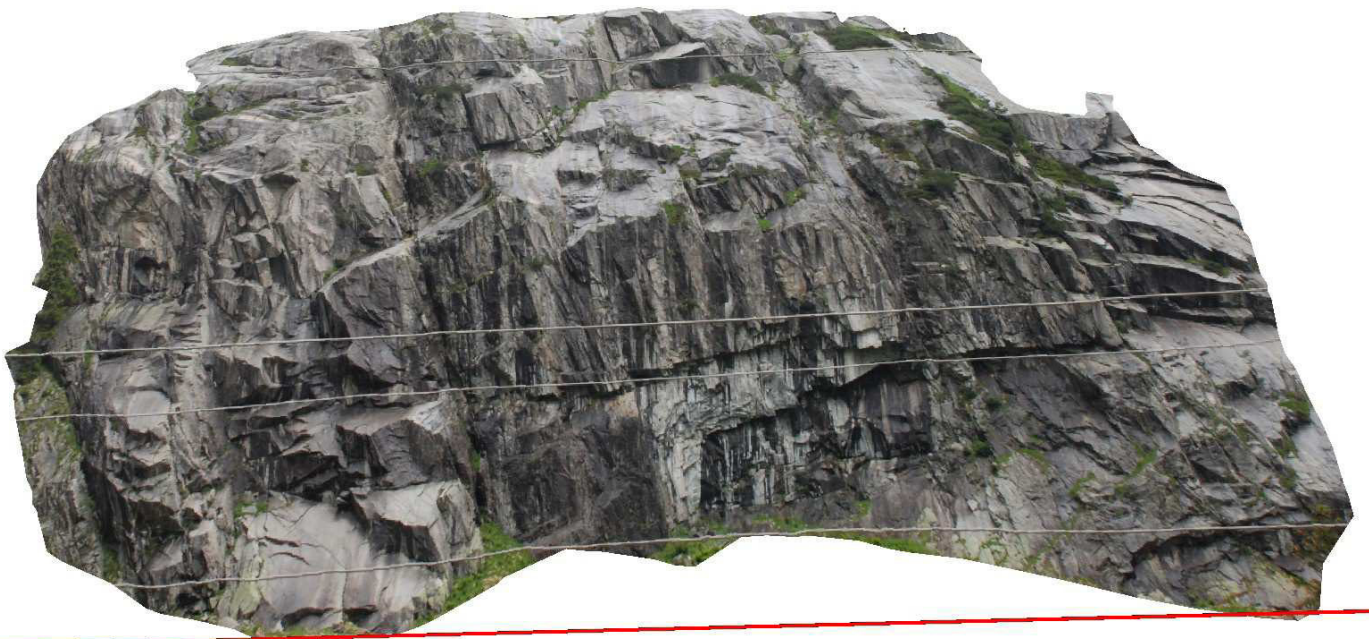
Figure 55 – Example of photogrammetric model with exfoliation joints of generation 2 (model n°9)
