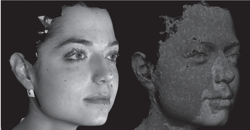
Fig. 4 - Three-dimensional reproduction of the facial soft tissues of a normal 20-y old woman obtained by a stereophotogrammetric instrument (three-dimensional image with texture, and polygonal mesh). Areas covered by hairs (eyelashes, head), and areas covered by other structures (lateral part of the face, below the mandibular angle) cannot be completely identified by the system. The colour version of this figure is available at the JASs website.
