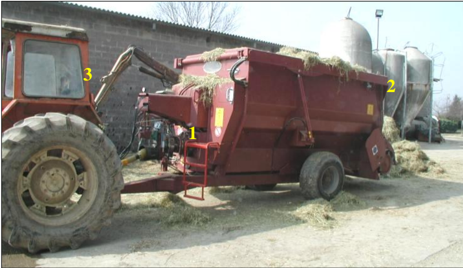
Figure 2. The 10 m 3 trailed horizontal-auger self-loading feed mixer wagon used for the farm tests; 1) limiter device; 2) sensors for the loading arms position; 3) the ECU positioned in a safe working place inside the tractor cab.
