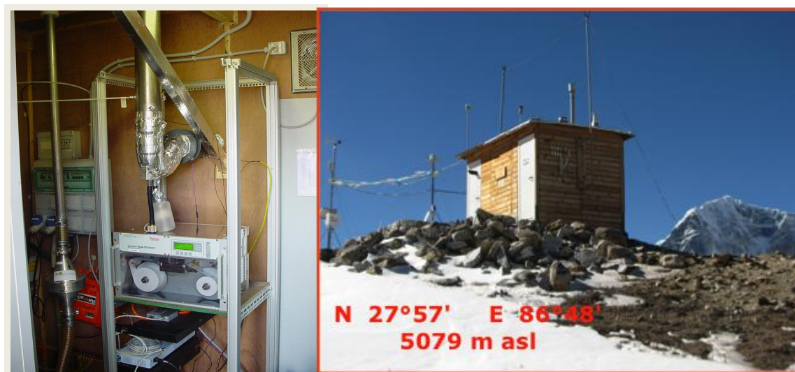
Figure 11: The NCO-P Station and the aethalometer for BC monitoring
