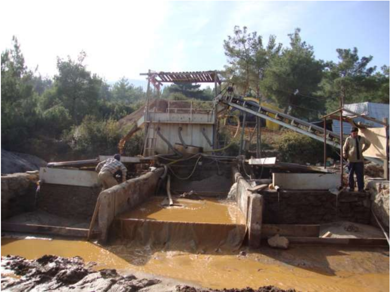
Fig. 11. Panoramic view of the enrichment plant with shaking tables in the foreground and jig in the background.
