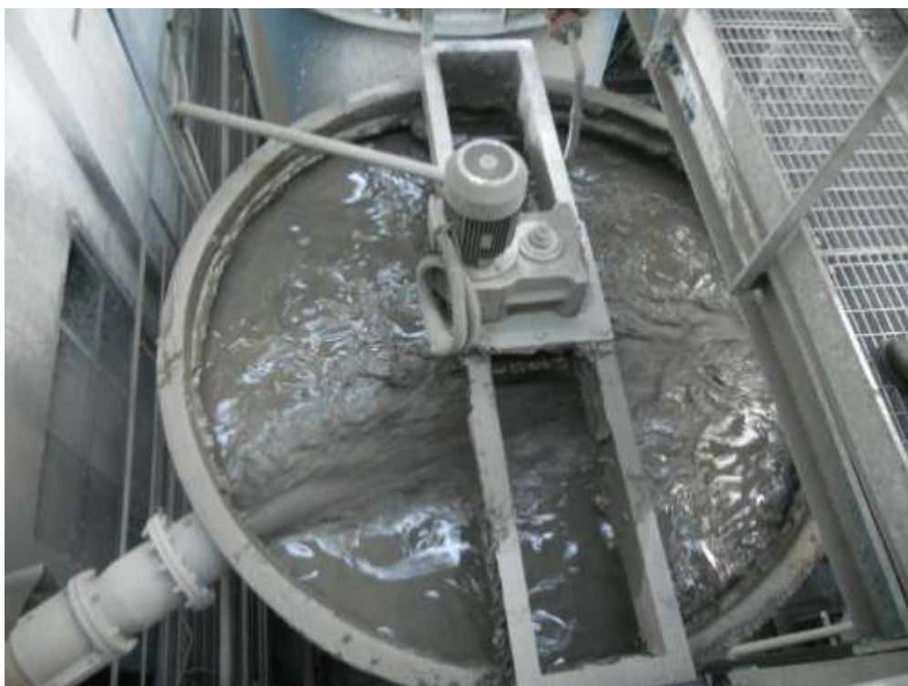
Fig.52 Picture of a flotation enrichment cell of copper ore, Fusharrez.
