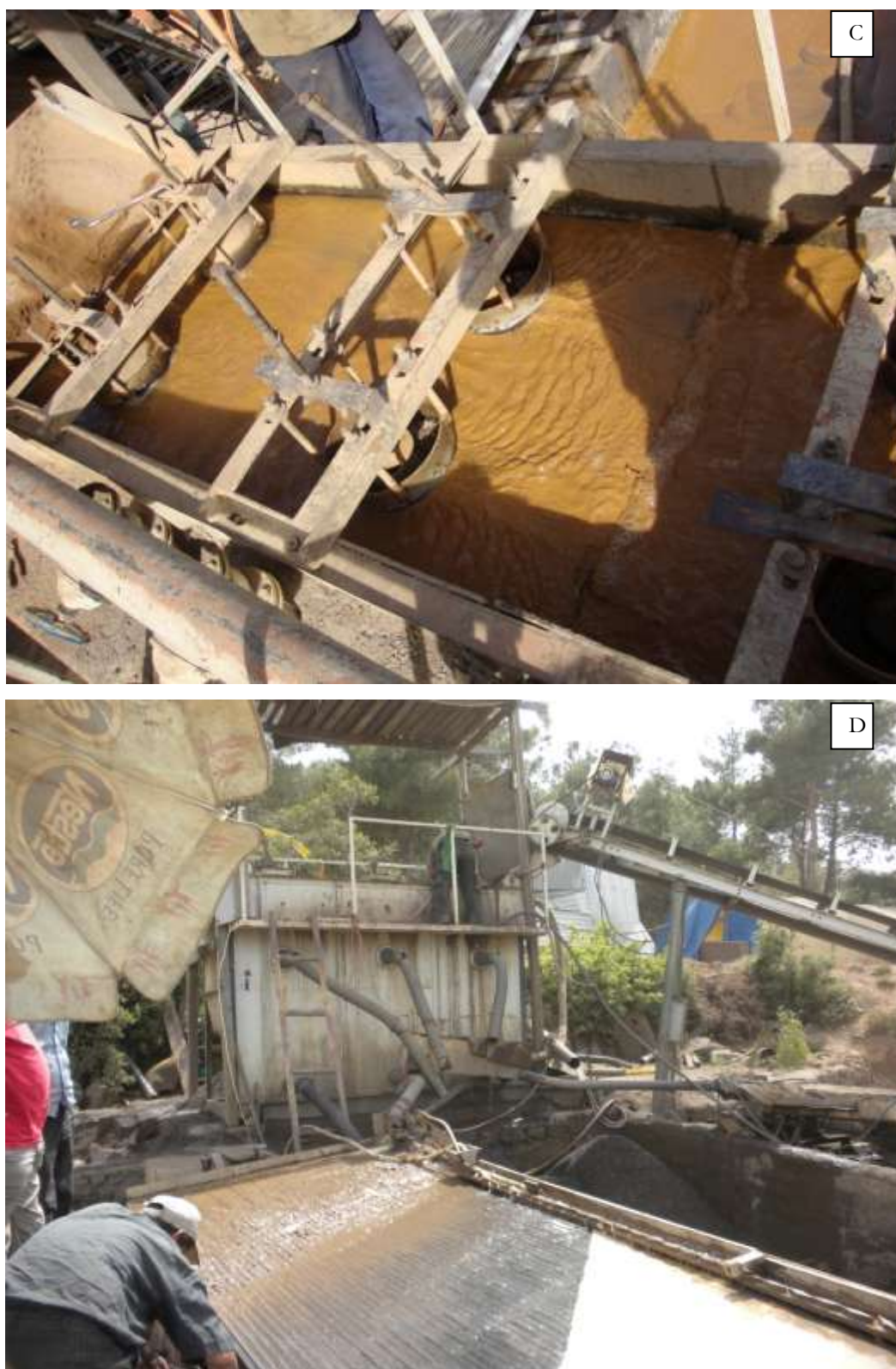
Fig 13. Pictures of manganese enrichment plant: A- comminution devices with jaw crusher, sieves and ball mill, B- Frontal view of enrichment devices with shaking tables and jig, C- View of the jig from the top, D- shaking table 1.
