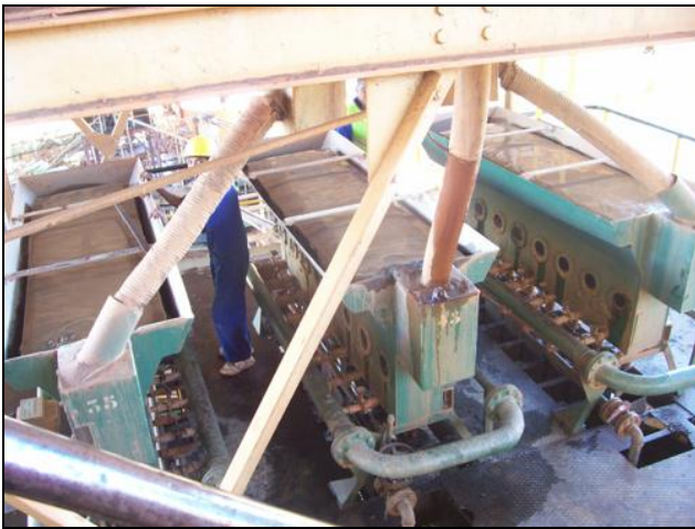
Figures 8 & 9. Hydrosizers (on the left) and series of shaking tables (on the right) at Brieville enrichment plant.
