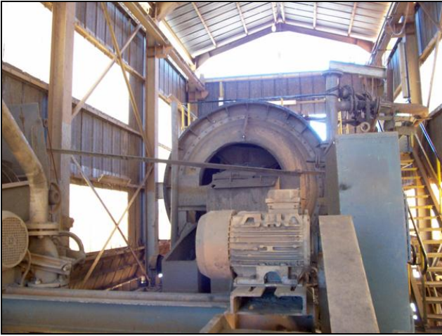
Figures 6 & 7. Tumbling ball mill (on the left) and vibrating screen (on the right) at Brieville enrichment plant.
