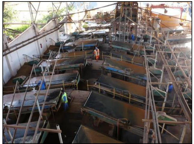
Figures 8 & 9. Hydrosizers (on the left) and series of shaking tables (on the right) at Brieville enrichment plant.
