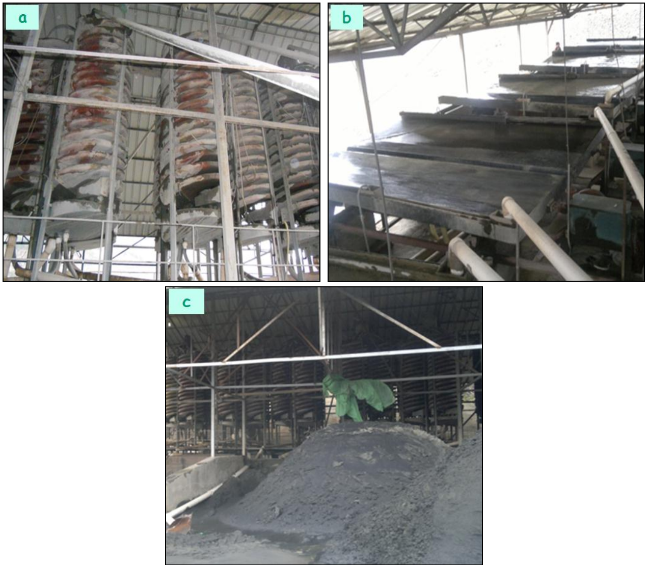
Figure 6. Photos taken at Krasta enrichment plant. (a) Spirals. (b) Shaking tables. (c) Stock of chromite concentrate sand.
