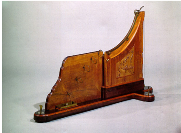
Fig. 5 Instrument to demonstrate free fall (along a parabolic trajectory) from the Museum of Science of the University of Coimbra Physics Collection (Cabinet for Experimental Physics, created in 1773)
