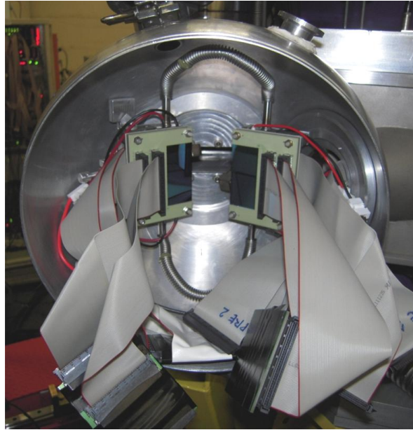
Fig. 3.9 - Photograph of the TRACE telescopes inside the scattering chamber; only the back contact of the \Delta E detectors is visible. The high-density flat cables are also visible, in grey, as well as the pipes for the cooling system. The adapters of Fig. 3.7 can be seen at the bottom, covered in insulating black tape.
