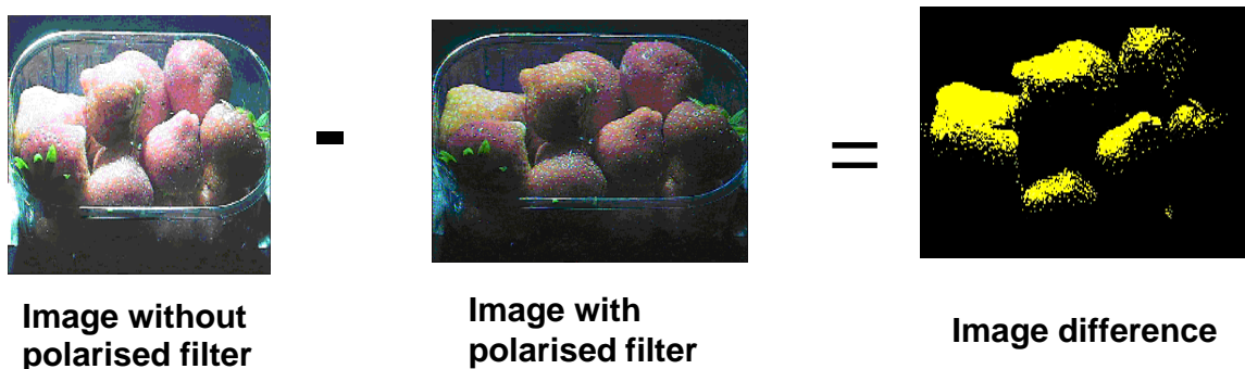
Fig.10 - Three images used to obtain a brightness index (IB) to sorting the strawberries basket for brightness.
