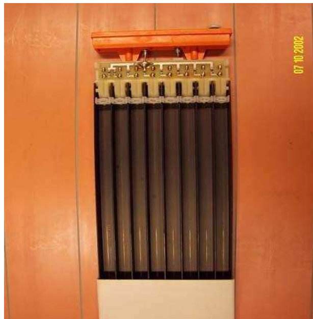
Figure 3.19: Sketch of an 8-cell module (top), and photo of an LST partially inserted in the sleeves (shown at the bottom of the picture).
