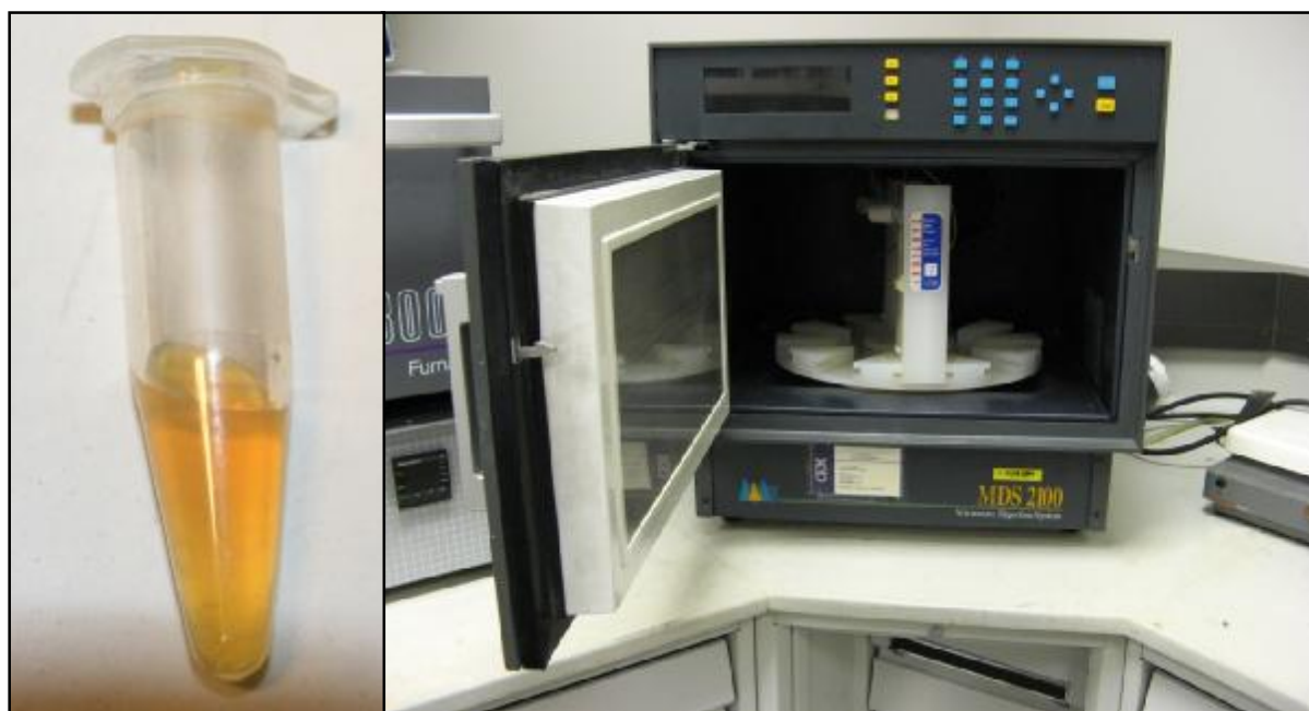
Figure 2. On the left, the Ag colloid obtained by microwave-supported glucose reduction of silver sulfate in the presence of sodium citrate as a capping agent. On the right, the CEM MDS-2100 microwave digestion system with a pressure resistant Teflon microwave vessel where the nanoparticle synthesis is carried out. Photographs taken by dr. Marco Leona.
