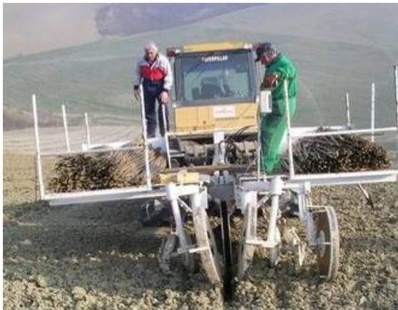
Figure 4 : Planter machine for MRF plantations coupled with tractors, plant rods are loaded on the platform near to the operators.
