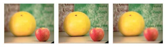
Figure 2.10: Three images captured with different focal length
