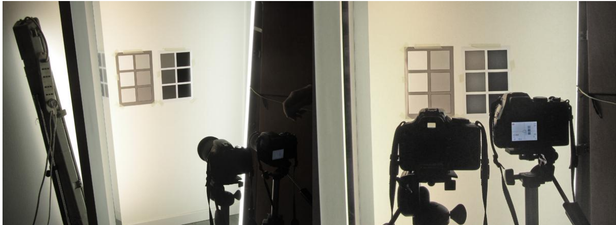
Fig. 40: the patches are visible on the wall. The fluorescent lights are placed vertically all around. The two cameras are used in the same time to take the pictures.
