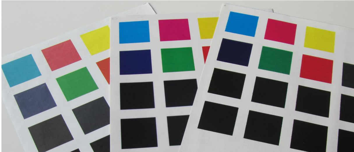
Fig. 86: Some of the patches used in the learning phase. From left to right: blueback paper, sticky paper, PVC canvas
