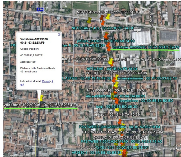
Figure 6: The APs observed on field (orange) vs. the APs reported in the database (yellow)
