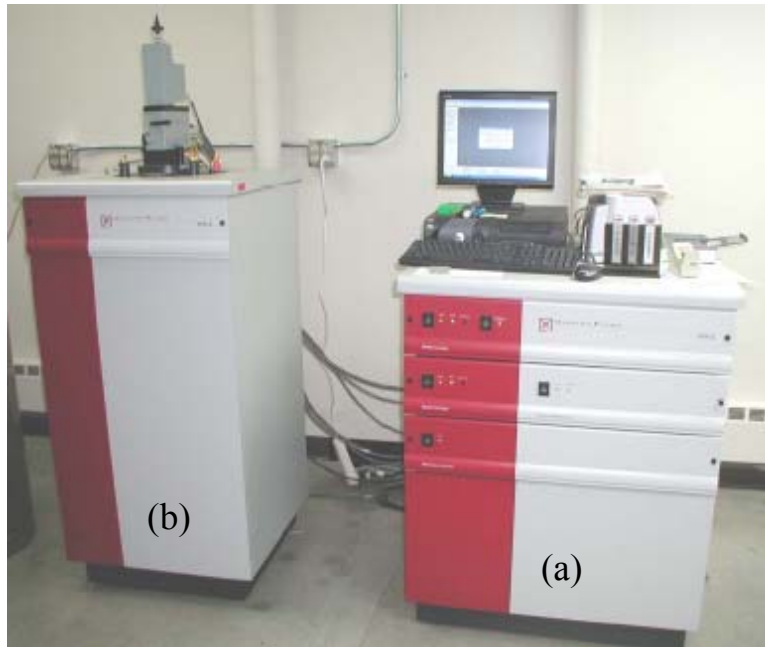
FIG. 3.4 Magnetic Property Measurement System (MPMS) XL; (a) computer and cabinet for gas handling and all control electronics, (b) cabinet for dewar.
