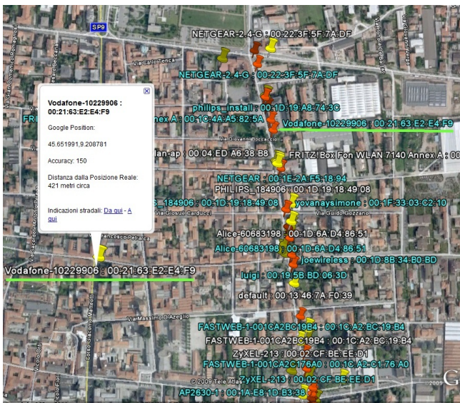
Figure 2: The APs observed on field (orange) vs. the APs reported in the database (yellow)
