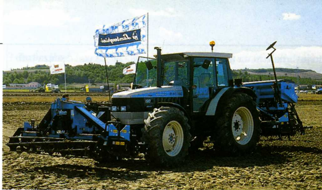
Fig. 5 - Aratro a dischi "offset" rainato, con organi lavoranti diversi sui due assi Trailed "offset" disc harrow, with different types of discs on the two axles
