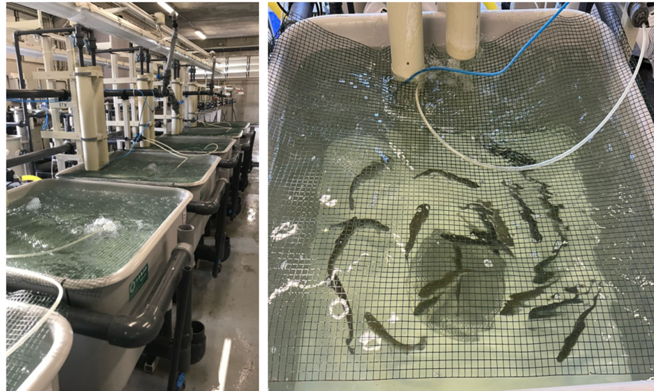
Figure 1. Lateral and front views of the experimental tanks. Water re-entered each tank via two lines: one passing through an oxygenator (longer tube, blue pipe = O 2 supply) and the other through a degasser (shorter tube). Each tank was also equipped with an aerator (white pipe = air supply).
