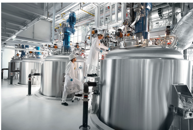
Figure 1. New fermentation reactors for the production of penicillin in Kundl, Austria. [Reproduced with kind permission, from Ref.18].
