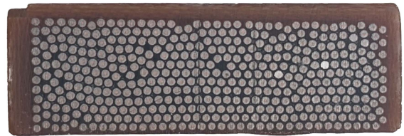
Fig. 3. Picture of a scrapped MCTSXF cross-section showing single insulated wire in silver, epoxy in dark brown and coil insulation in light brown.
