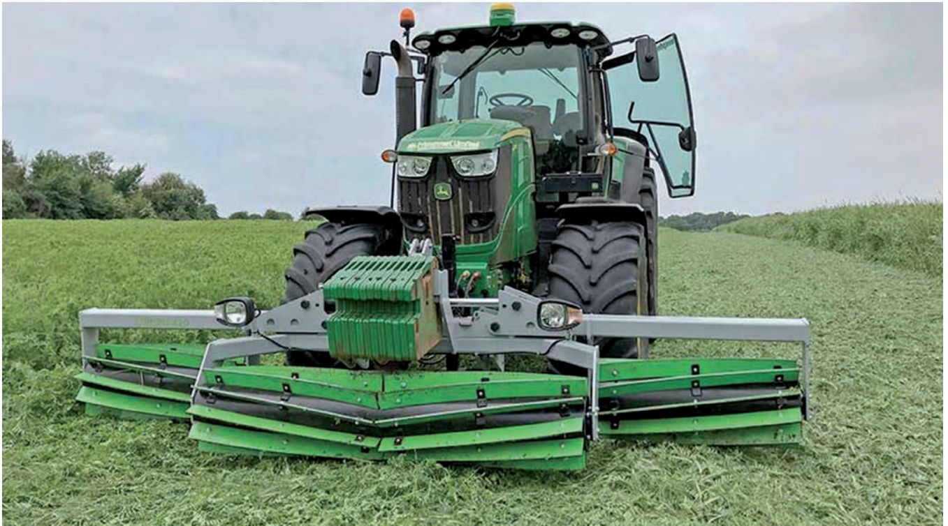
Rullo crimper portato anteriormente. (Fonte: https://www.fwi.co.uk ) Crimper roller carried in front (Fonte: https://www.fwi.co.uk )
