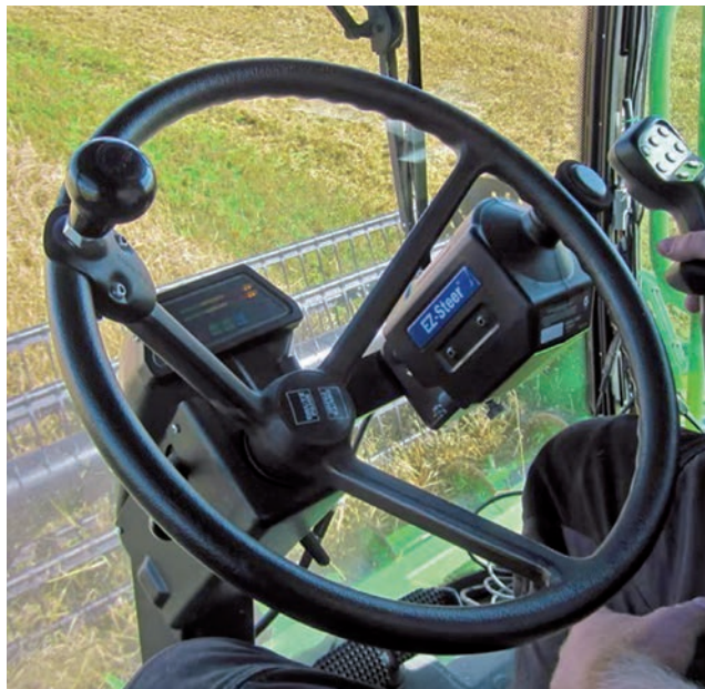
Sistema di guida semi-automatica con attuatore al volante (cortesia: https://agriculture.trimble.com ) Semi-automatic steering system with steering wheel actuator (courtesy: https://agriculture.trimble.com )
