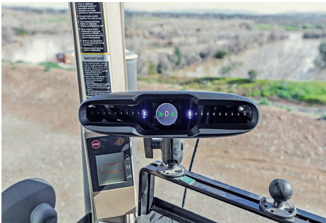
Interfaccia di guida assistita con barra a led (cortesia: www.topcompositioni ng.com ) Assisted guidance interface with led bar (courtesy: www.topcompositioni ng.com )
