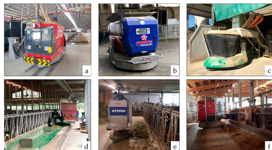
Figure 4. Different models of AFS wagons: wheel-driven (a); self-propelled (b,c,f); rail-suspended chopper-mixing and distributor (d); rail-suspended distributor (e). Pictures taken by the authors.
