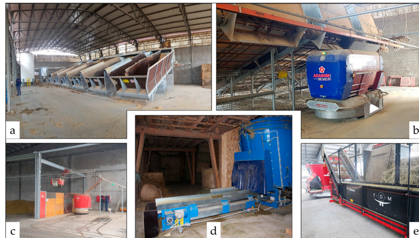
Figure 3. Different types of kitchens. Kitchen with temporary storage containers (a,b,e); self-loading crane experience (c); fixed mixing with belt conveyors (d). Pictures taken by the authors.
