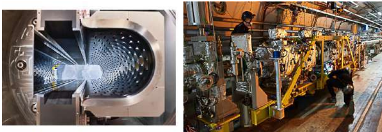
Fig. 3. The cross-section of one of the new TDIS modules is shown on the left: the graphite jaws have to intercept any vertically mis-kicked beam while the counter-rotating beam circulates unperturbed, in the same vacuum tank, to the side of the jaws. The TDIS installed in IR8 of the LHC is also shown on the right.
