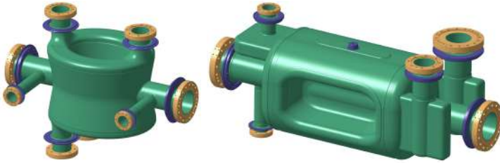
Fig. 3. Schematic view of the cavity with interfaces (left) DQW; (right) RFD.
