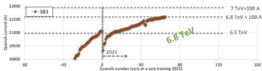
Fig. 10. Circuit current as a function of number of (re-)training quenches in LHC sector 81. During Run 2, the machine was operated at 6.5 TeV, while the 2021 commissioning campaign pushed the sector to achieve the 6.8 TeV energy equivalent.
