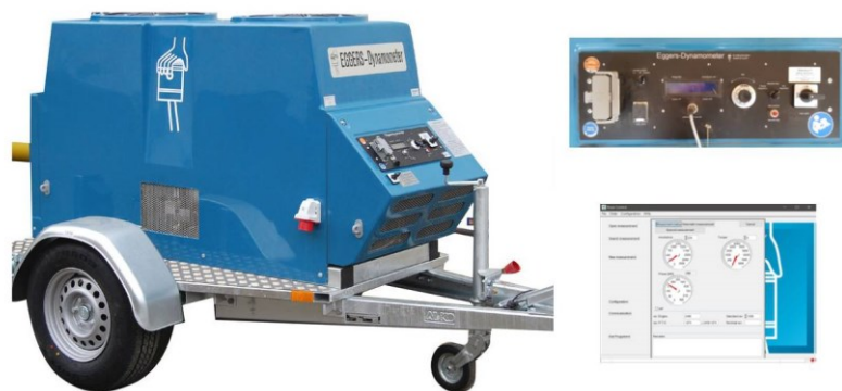
Fig. 2. Left: the wheeled electromagnetic dynamometer Eggers-Dynamometer PT 301 MES (KL-Maschinenbau GmbH Rendsburg - Germany). Right: the control panel located on the device (top) and the screen of the control through the computer, via Bluetooth (bottom).
