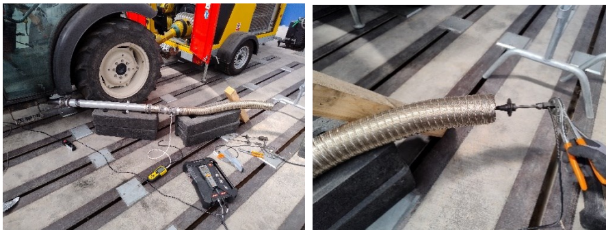
Figure 2: in order to measure the emissions level, a pipe was inserted in the exhaust gas line, including the probe of the flowmeter, and those of the gas analyzer and smoke tester.
