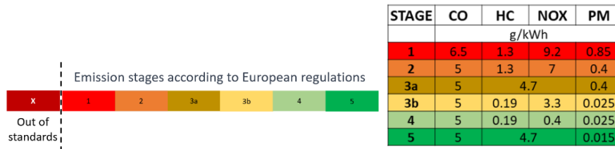
Figure 3: the "traffic light colour logic" was adopted to better understand, at a glance, the amount of gaseous pollutants recorded compared with the standard limits
