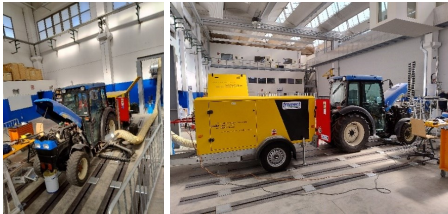
Figure 1: the tested tractor New Holland TN70VA was connected to a dynamometer Froment Sygma 50, to measure its performance
