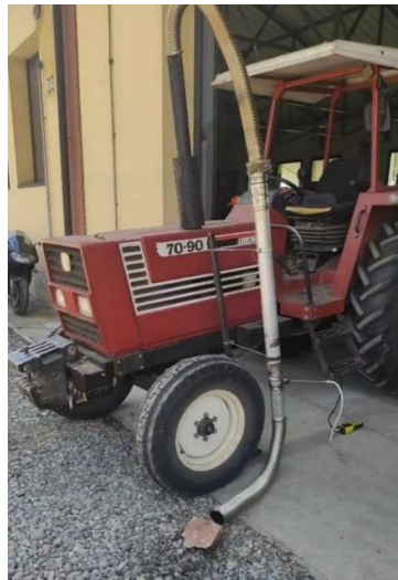
Fig. 1. To measure the gas flow, the Fiat 70-90 exhaust terminal was linked to a bypass pipe.
