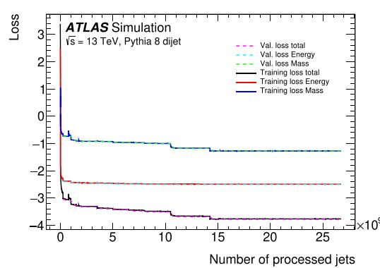
**Figure 3.** The loss evolution for the training (plain lines) and validation (dotted lines) data samples. The different spikes and drops correspond to the transitions between training steps (see table 3) and are due to the variations of the loss function.
