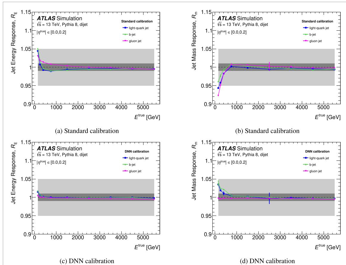
**Figure 12.** Jet energy (left) and mass (right) responses versus  $E^{\text{true}}$  for different jet flavours, calibrated with the standard calibration (a), (b) and the DNN calibration (c), (d). The horizontal bands represent 1% (dark) and 5% (light) up and down divergences from closure.
