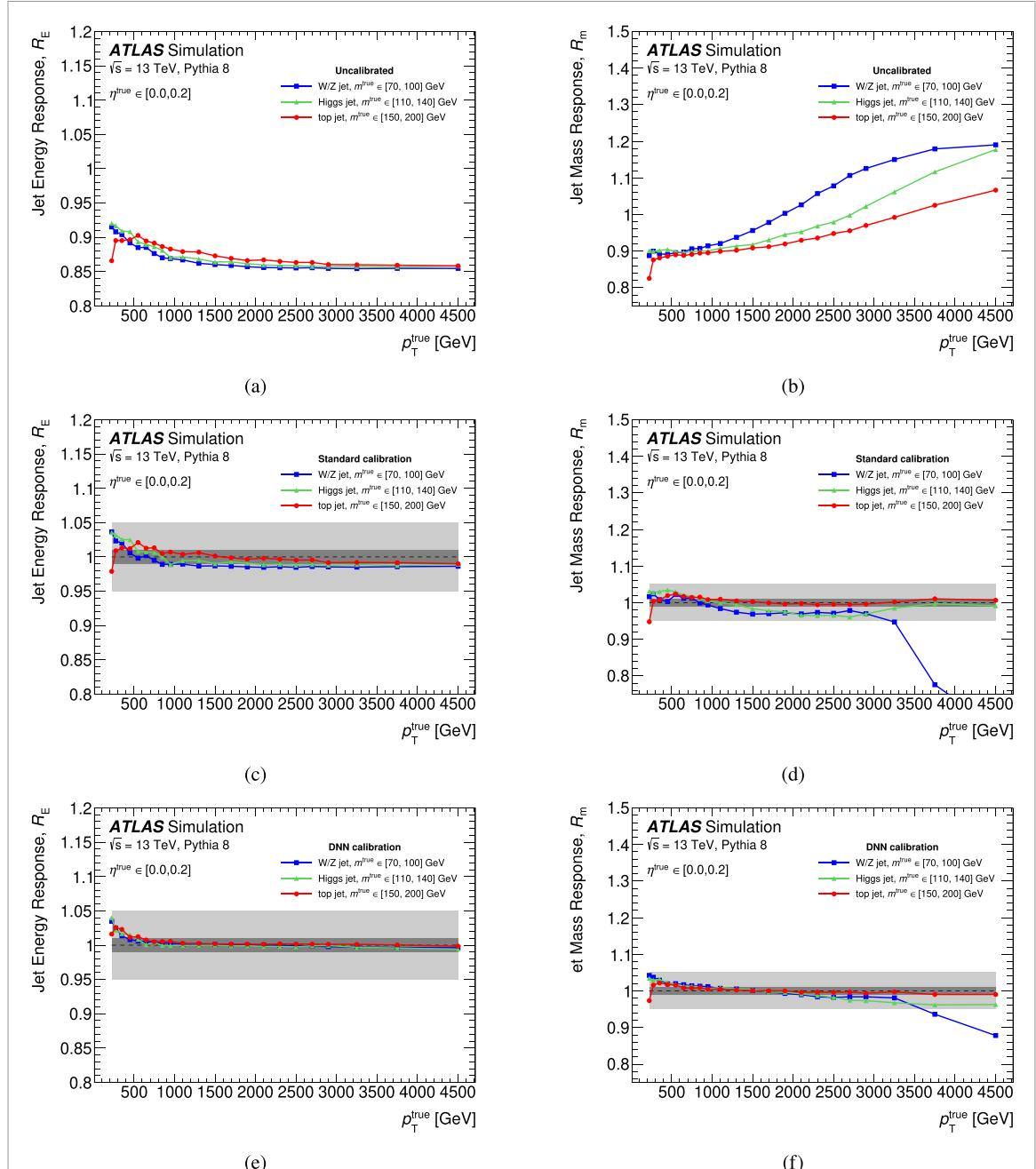
**Figure 8.** Boosted  $W/Z$ , top-quark and Higgs boson jet energy (left) and mass (right) responses as a function of  $p_T^{\text{true}}$  for different calibrations: (a), (b) no calibration, (c), (d) standard calibration and (e), (f) DNN calibration. The horizontal bands represent 1% (dark) and 5% (light) up and down divergences from closure.
