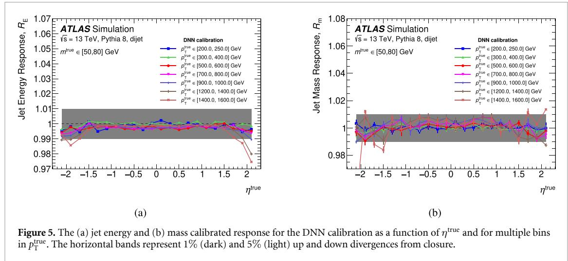
**Figure 5.** The (a) jet energy and (b) mass calibrated response for the DNN calibration as a function of  $\eta^{\text{true}}$  and for multiple bins in  $p_T^{\text{true}}$ . The horizontal bands represent 1% (dark) and 5% (light) up and down divergences from closure.
