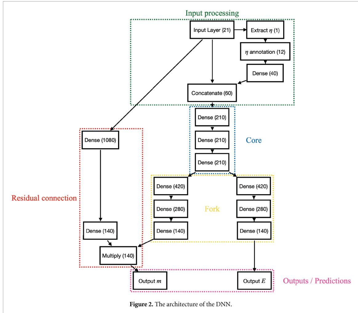
Figure 2. The architecture of the DNN.
