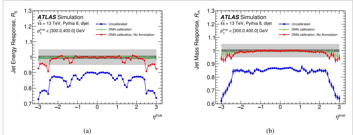
**Figure 6.** The (a) jet energy and (b) mass response before calibration (squares) and after the DNN calibration with (triangles) or without (circles) the  $\eta$  annotation step as a function of  $\eta^{\text{true}}$ . The horizontal bands represent 1% (dark) and 5% (light) up and down divergences from closure.
