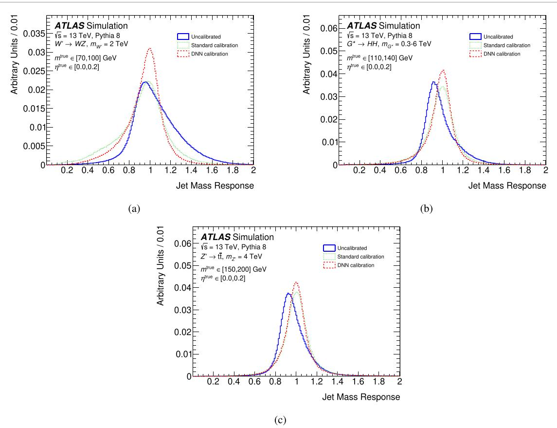
**Figure 7.** (a) Boosted  $W/Z$ , (b) Higgs boson and (c) top-quark mass response distributions (normalised to unity) for different calibrations: uncalibrated (plain line), standard calibration (dotted line) and DNN calibration (dashed line).
