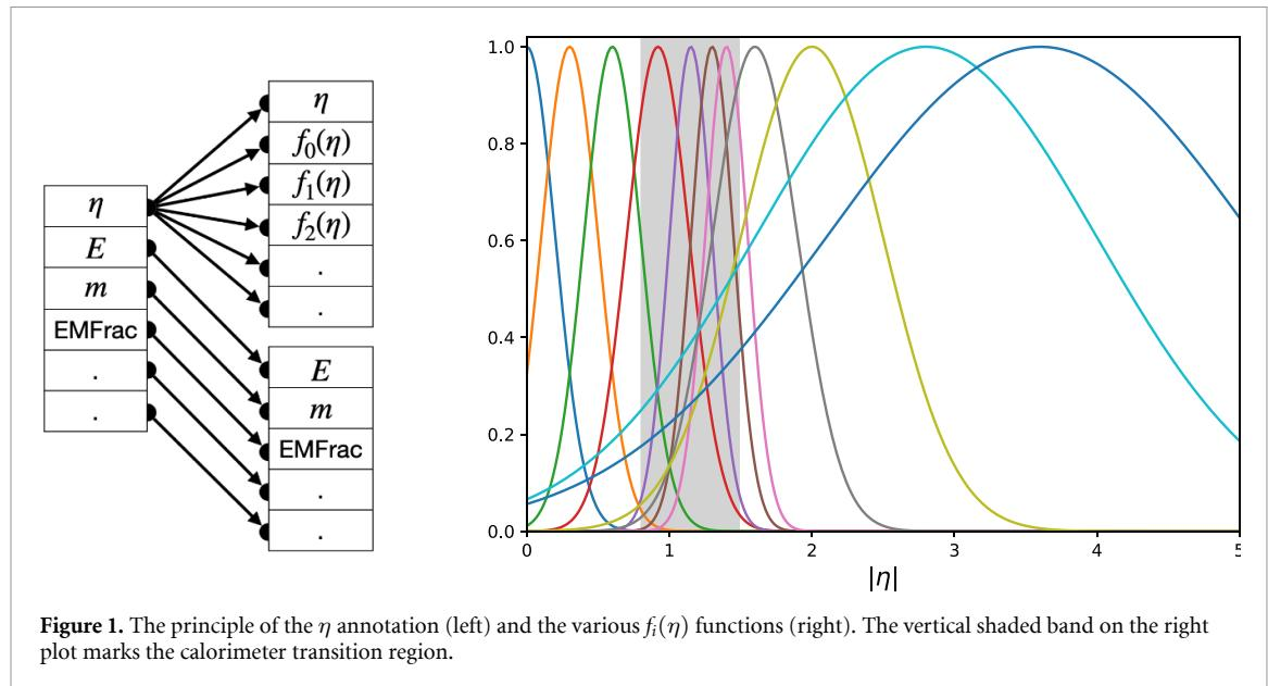
**Figure 1.** The principle of the  $\eta$  annotation (left) and the various  $f_i(\eta)$  functions (right). The vertical shaded band on the right plot marks the calorimeter transition region.
