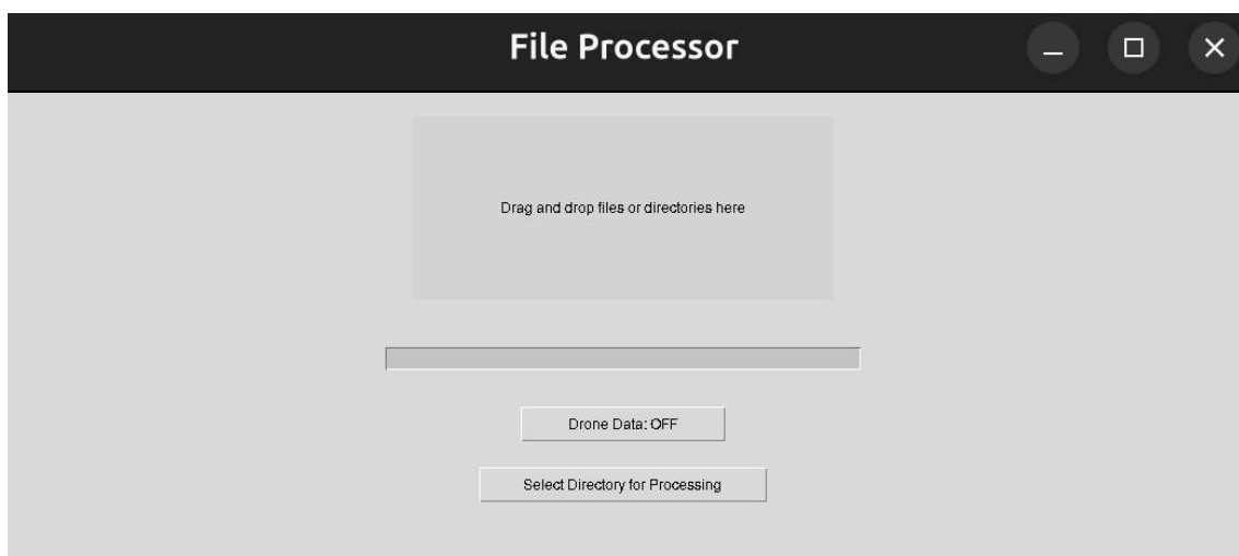
Figure 4.4: Graphical user interface of the inspection tool. Users can drop files or select a folder containing .las point cloud files for processing. The progress bar indicates the current status of the pipeline. Once finalized, a .las file is produced with the same name, only with a _segmented suffix added and an additional column with the segmentation results named classification . The "Drone Data" toggle allows users to specify whether the input corresponds to TS40K (helicopter-mounted LiDAR) or TS-RGB (UAV-captured LiDAR).
