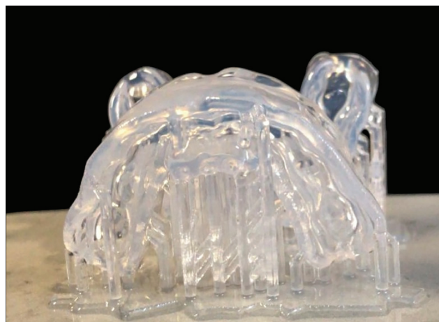
FIG. 2. The 3D printing of the appliance according to the digital dental set-up performed by the orthodontist
