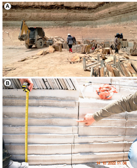
Figure 2. (A) Mining front of laminated limestone from the Crato Formation in the Nova Olinda Quarry (see location reported in Table 1). (B) Appearance of the “sete cortes” bed on the mining front in the Nova Olinda Quarry. Note the cut lines separating 10 cm thick slabs.
