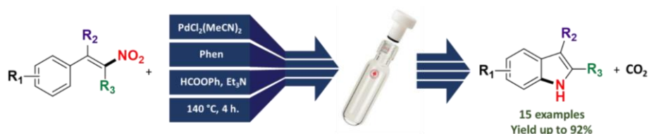
Figure 1: Schematic Representation of Synthesis of indoles from \beta -nitrostyrenes using HCOOPh as a CO surrogate.
