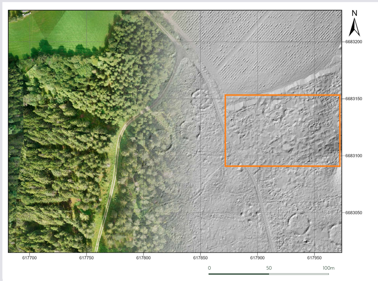
Figure 43: Aerial photograph fading into a hillshaded DTM of a wooded area in Norway showing multiple circular charcoal kilns. Triangular artefacts created by interpolation across areas where no ground points were recorded can be seen highlighted in the orange area in this image (credit: Magnar Mojaren Gran, NTNU University Museum)
