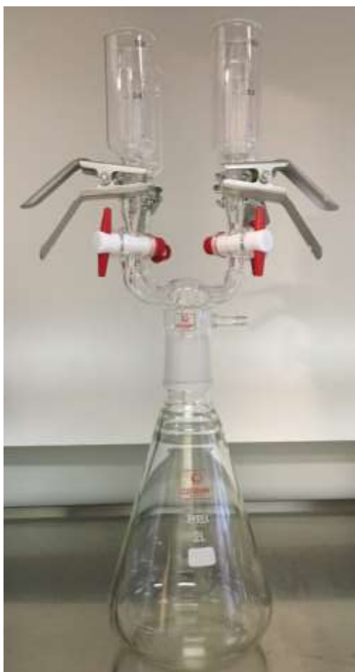
Figure S2. In-house manufactured glass filtration apparatus allowing to filter up to four samples simultaneously and valves to individually regulate vacuum. The setup consists of the following components; four open reservoir flasks that are mounted on top of four extension of a filtering head placed on top of a conical flask, which collects the sample liquids. Each of the four extensions has a porous plate on which the filter is seated and a closing valve below to individually regulate the vacuum. The tube of the vacuum pump is attached to an extended glass tube at the lower part of the filtering head. Metal clamps hold the reservoir flask and filtering head together and can be detached in order to remove the filter membranes.
