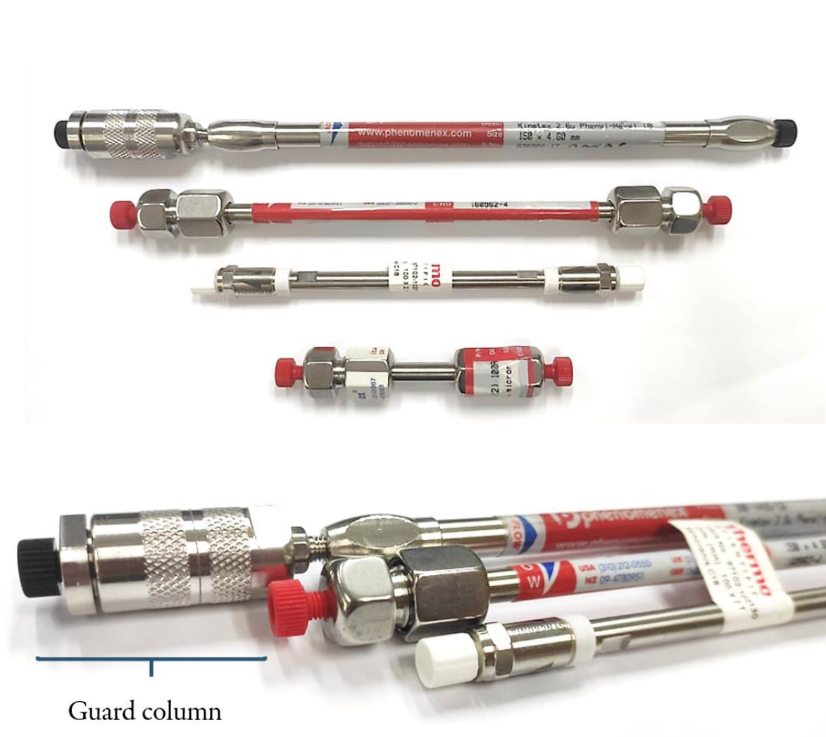
Figure 2. Examples of packed columns employed in HPLC analysis. In the detail, a guard-column is shown. The guard-columns help preserving the analysis column by removing particulate contaminants and highly absorptive compounds from samples, prolonging column life. Columns represented in the photo were provided by Phenomenex (Torrance, California, USA) and Thermo Fisher Scientific (Waltham, Massachusetts, USA). Photo by Annalaura Lopez.
