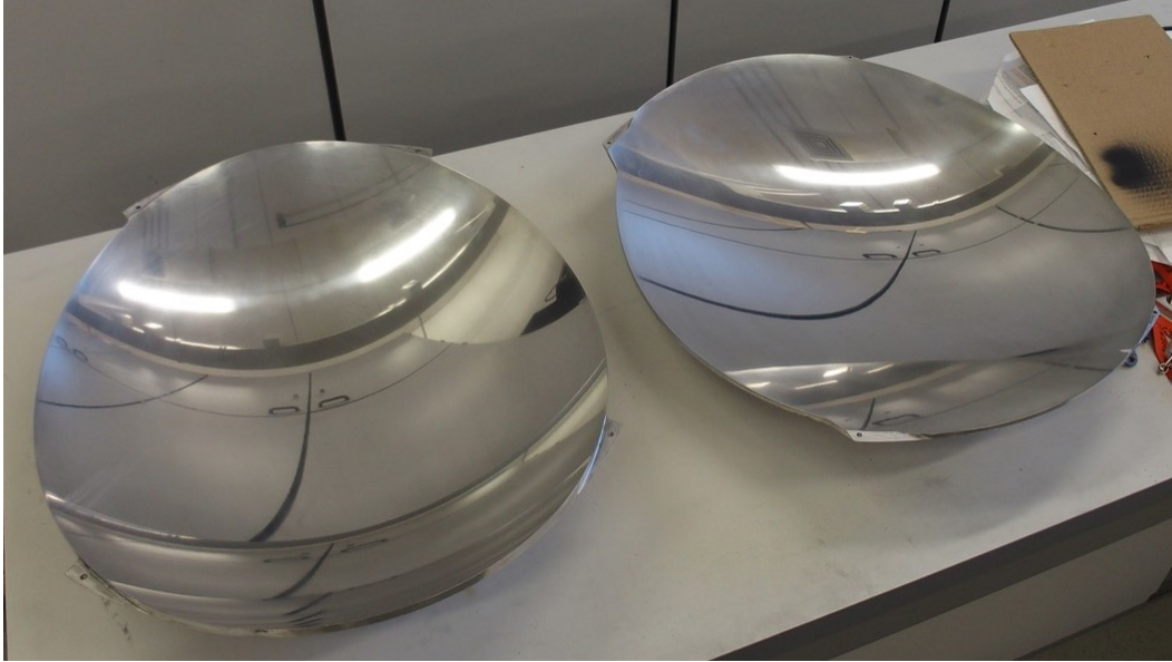
Figure 15. The two mirrors of the FI combiner during the manufacturing procedure, before the final polishing step.
