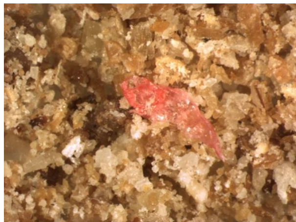
Figure 3. Example of image of feed sample and a piece of red/transparent packaging material, obtain with the use of stereomicroscope and high-resolution CCD camera (CoolSNAP-Pro colour camera).
