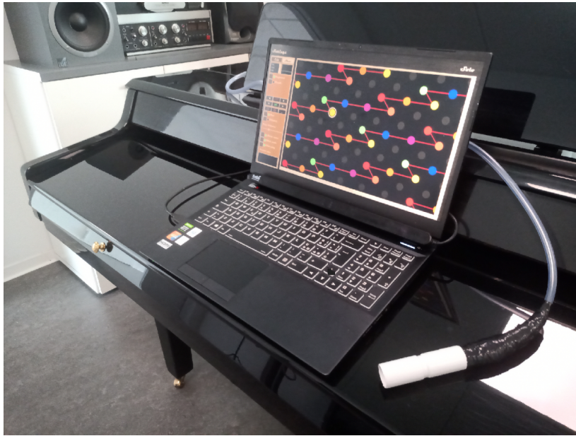
Figure 9.1.: The latest version of Netytar running on a laptop having NeeqBS breath sensor peripheral connected.
