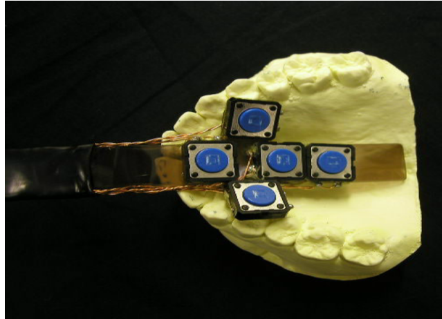
Figure 5.2.: The PET board placed on the palate in Niikawa’s Tongue-controlled Electro-musical Instrument.
