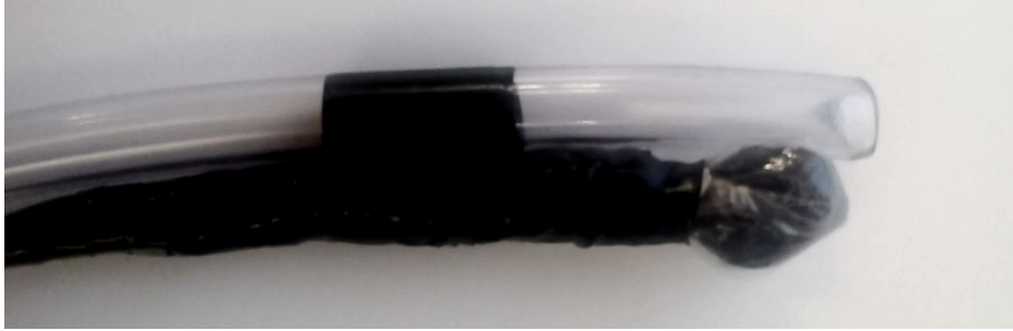
Figure 11.2.: Resin's mouthpiece, consisting of the sound tube and the Lavalier microphone.
