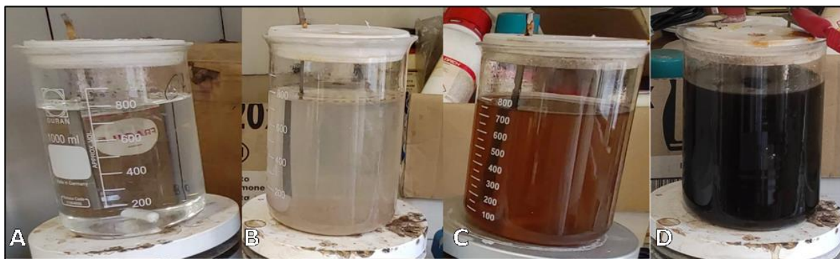
Figure 122: Ammonium chloride solution with manganese before electrolysis, A, and after 5, 15, 60 min, B, C, D.
