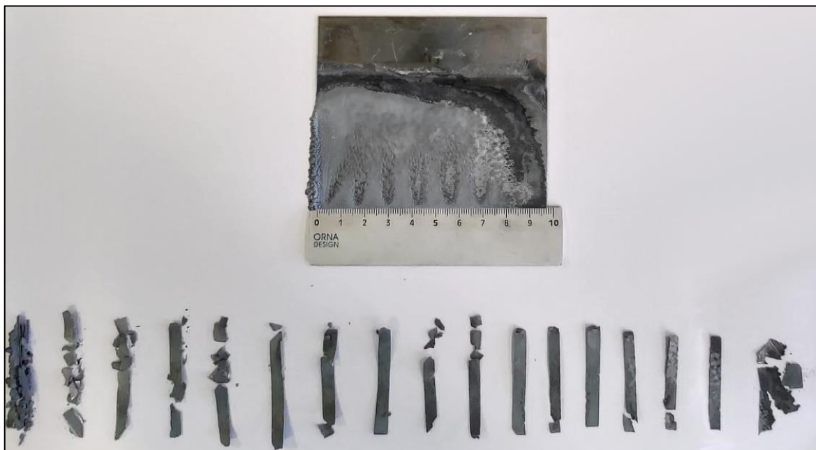
Figure 205 Zinc plate cut in 5 mm strips for current density distribution analysis.
