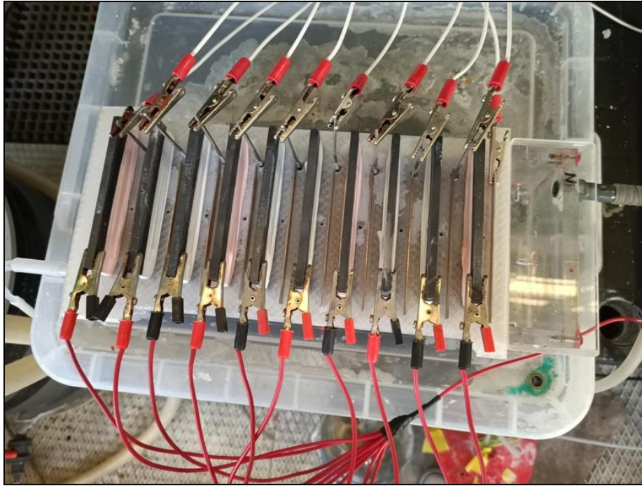
Figure 45: Snake path electrodeposition cell, top view.
