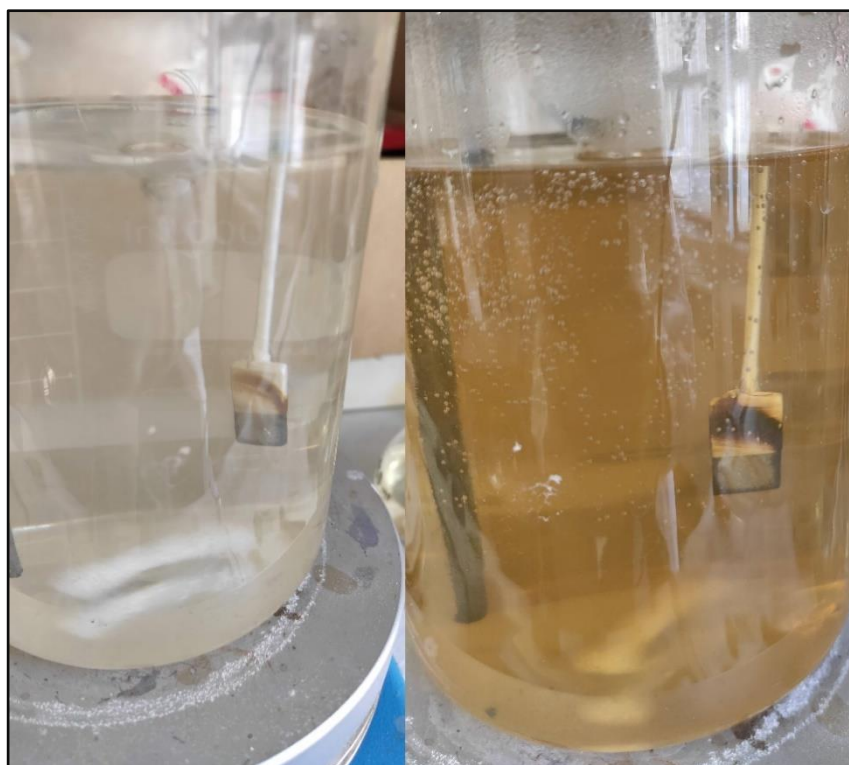
Figure 123: Detail of titanium activated electrode during the first minutes of electrolysis in presence of manganese.
