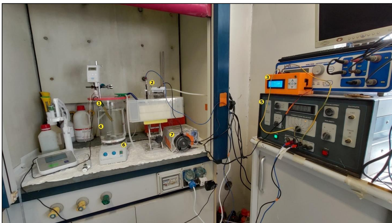
Figure 138: Experimental setup. 1-pH electrode, 2-Hull cell, 3-Potential logger, 4-Recirculating tank, 5-Potentiostat, 6-Heating plate, 7-Peristaltic pump.
