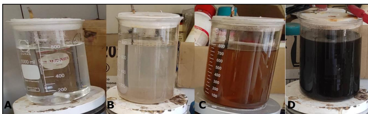
Figure 52: Ammonium chloride solution with manganese before electrolysis, A, and after 5, 15, 60 min, B, C, D.
