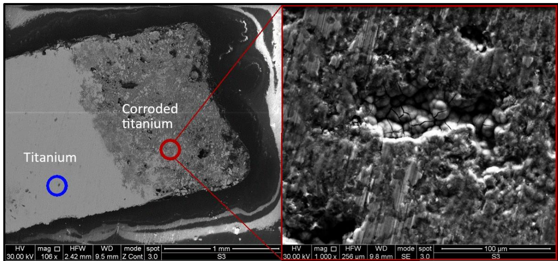
Figure 132: Corroded titanium anode cross section and magnification of the corroded structure.
