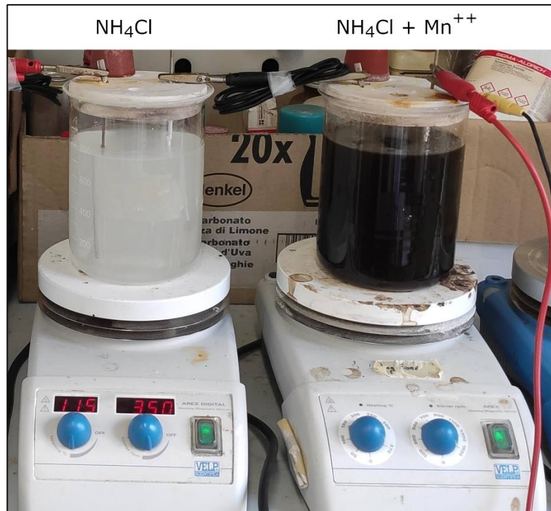
Figure 124: Solution appearance after 1 hour of electrolysis.
