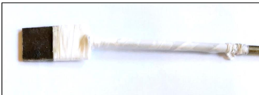
Figure 120: Activated titanium electrode prepared for tests
