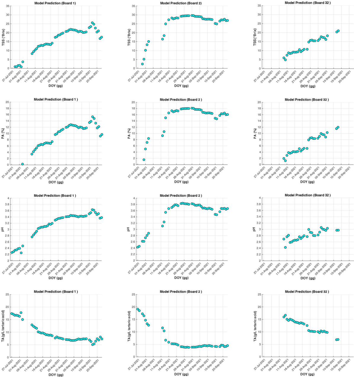
Figure 4.13 Optical prediction (TSS, PA, pH and TA) from field sensors (board 1, board 2, board 32) from the campaign 2021.
