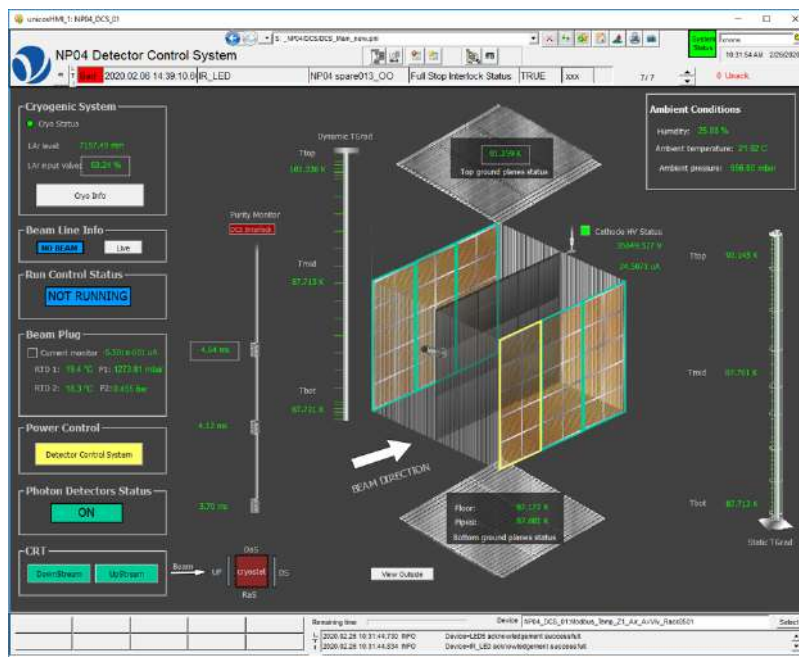
Figure 84. The DCS overview display, showing the color-coded status of the detector components, the average temperatures on the two T-gradient rods, and the most recent electron lifetime measurements.
