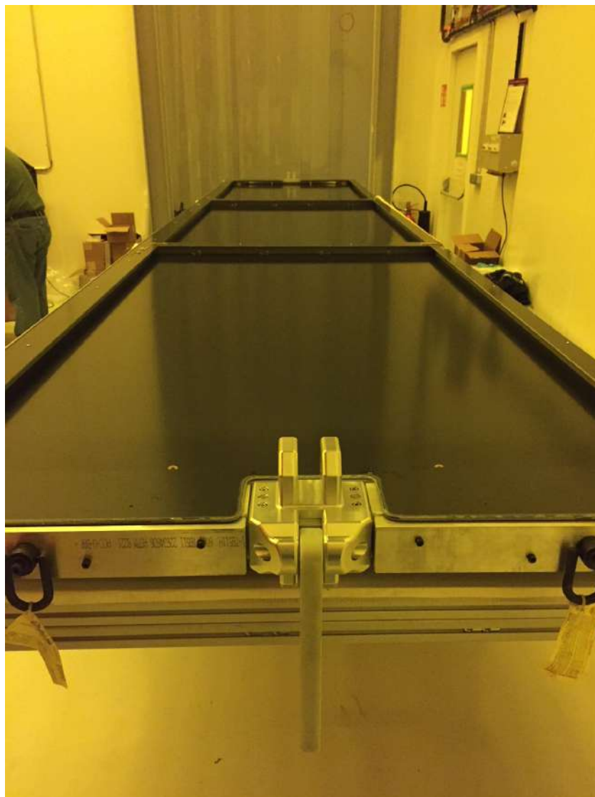
Figure 16. Completed 6 m long ProtoDUNE-SP CPA panel on the production table.
