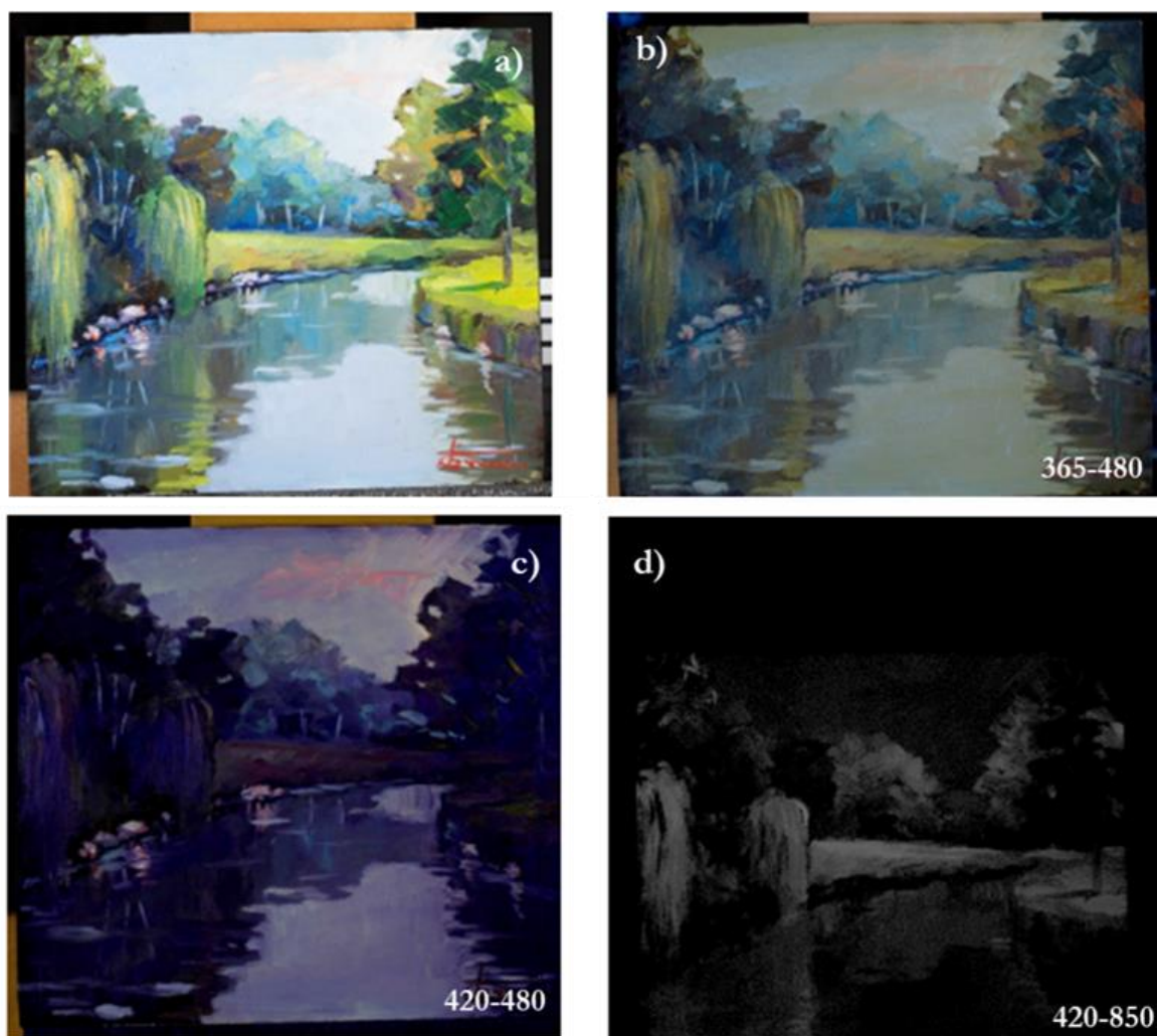
Figure 29. a) Visible image of the painting Addetta near Zoate by G. Faraone; b) UVF image; c) VIVL image (excitation source 420 nm); d) VIL image (excitation source 420 nm).
