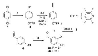
Scheme 1. Reagents and Conditions: (a) pentafluoropyridine,  $K_2CO_3$ , ACN, 25 °C, 12 h; (b) trimethylsilylacetylene, Pd(PPh<sub>3</sub>)<sub>4</sub>, PPh<sub>3</sub>, CuI, TEA, 90 °C, 3 h; (c) TBAF, THF, -78 °C, 5 min; (d) *N*-bromosuccinimide, thioacetamide, ACN, 25 °C, 2 h; (5a) or AgNO<sub>3</sub>, I<sub>2</sub>, MeOH, 25 °C, 24 h (5b).
