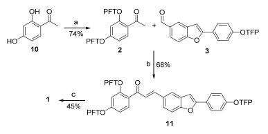
Scheme 2. Reagents and Conditions: (a) pentafluoropyridine,  $K_2CO_3$ , ACN, 25 °C, 12 h; (b) trimethylsilyl trifluoromethanesulfonate, triethylamine, DCM, -20 °C to 25 °C, 12 h; (c) methyl thioglycolate, KF, 18-C-6, ACN/H<sub>2</sub>O, 25 °C, 12 h.
