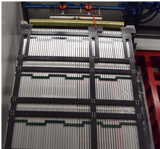
Figure 20. Endwall FC assembly, the stacked modules are visible. The endwall is hung in front of the cryostat before insertion through the TCO. The visible face is the one that will face the inside of the detector active volume. The dark grey FRP plates are the support structure of the endwall and interconnected between the volumes.
