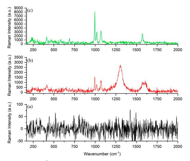
**Figure 9.** SERS spectra of  $10^{-3}$  M BT recorded on (**a**) macro-copper, (**b**) CuUWs, and (**c**) AgNSs@CuUWs ( $\lambda_{ex}$ = 785 nm, P = 15 mW, t = 3 × 20 s).
