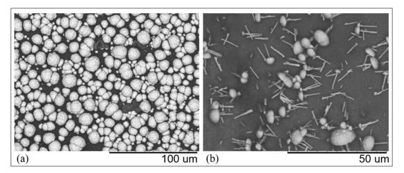
**Figure 6.** SEM images of the copper deposit obtained using track-etched PC templates onto a GC: (**a**) surface before etching; (**b**) mushroom-like nanostructures after etching in  $CH_2Cl_2$  for 1 min. Deposition at -0.400 V vs. Cu(pseudo ref) for 600 s; etching in  $CH_2Cl_2$  for 1 min.
