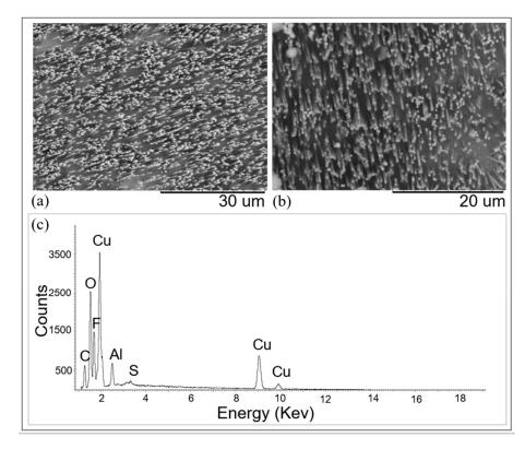
**Figure 7.** SEM images of CuUWs obtained using track-etched PC templates onto: (**a**) GC working electrode; (**b**) Cu working electrode. Deposition at -0.400 V vs. Cu(pseudo ref) for 140 s (**a**) and 180 s (**b**); etching in CH<sub>2</sub>Cl<sub>2</sub> for 1 min. (**c**) EDS spectrum recorded on the CuUWs obtained after template deposition (**a**).
