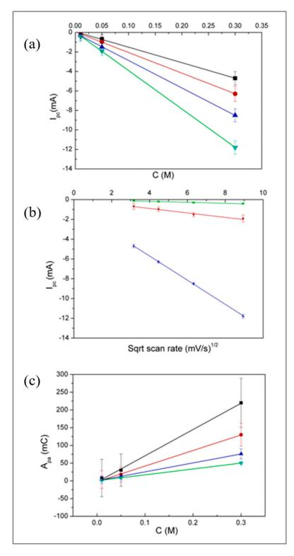
**Figure 5.** Plots obtained from data in Table 1, showing the dependence of: (a) cathodic peak current vs. CuSO<sub>4</sub> concentration, at scan rate: 10 (black); 20 (red); 40 (blue); 80 mV/s (green); (b) cathodic peak current vs. square root of the scan rate, at  $[Cu^{2+}]$ : 0.01 (green); 0.05 (red); 0.3 M (blue); (c) electric charge measured by integration of the anodic peak vs. CuSO<sub>4</sub> concentration at scan rate: 10 (black); 20 (red); 40 (blue); 80 mV/s (green).
