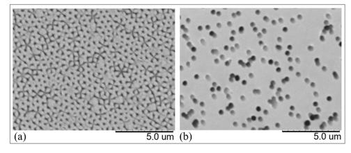
**Figure 1.** Scanning electron microscopy images of the surface of the membranes here used as templates: (**a**) anodized aluminum oxide; (**b**) track-etched polycarbonate.
