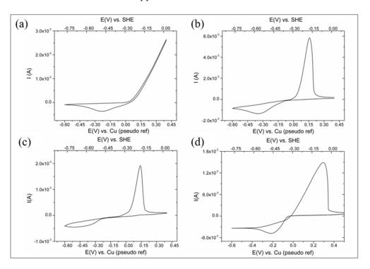
the oxidation of both the metallic copper deposited during the cathodic branch of the CV and the metallic copper that constitutes the electrode itself.
