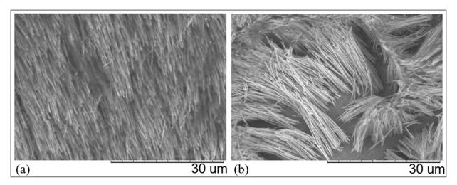
**Figure 8.** SEM images of: (**a**) self-standing, (**b**) collapsed CuUWs prepared by using a AAO template onto a Cu working electrode. Deposition at -0.250 V vs. Cu(pseudo ref) for 300 s; etching in 2 M NaOH for 5 min.
