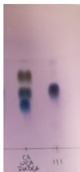
Figure 5.6: the TLC of the stereoinversion from cholic acid to ursocholic acid with the aid of Is2-SDR shows only ursocholic acid after less than one day (eluent: \text{CHCl}_3 :MeOH:AcOH=9:1:0.05, development reagent: Komarowsky's oxidizing solution). The reaction does not result to be reversible.
