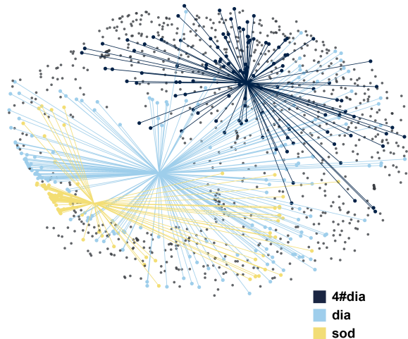
Figure 2 Geometric diversity within isorecticular groups of AB_2 MOFs. The graph shows a two-dimensional visualization of the cg-SOAP-based structural distances using an MDS embedding: generally, the closer two points are, the more similar their coarse-grained and re-scaled geometric structures. The distribution of the three most commonly occurring topologies within our dataset ( dia , sod , and fourfold-interpenetrated dia , denoted 4#dia ) is emphasized by lines that originate from the respective centroid. Dataset entries with different topologies than the three aforementioned ones are all represented by gray points.
